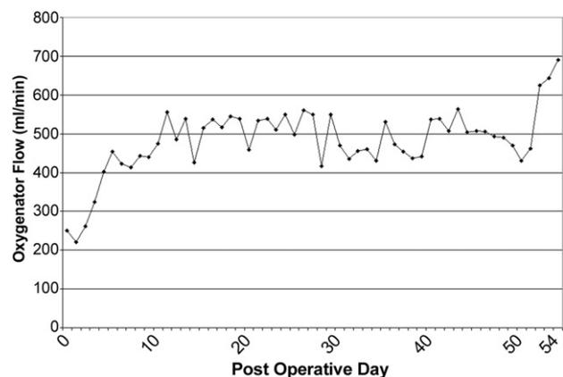
Fig 1. Flow through oxygenator recorded hourly with ultrasound flow meter.
