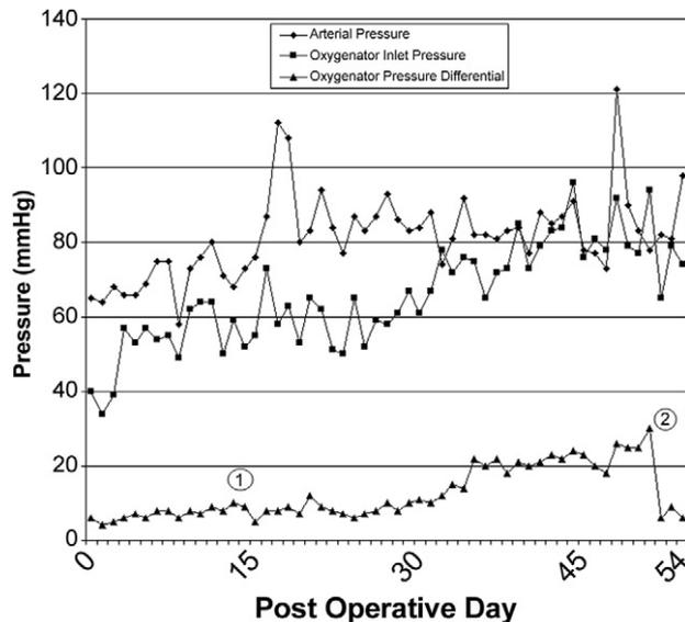
Fig 2. Measurements of arterial pressure, inlet oxygenator pressure, and pressure differential across oxygenator over the course of device support. The two oxygenator changes are marked by circled numbers adjacent to the pressure differential values.
